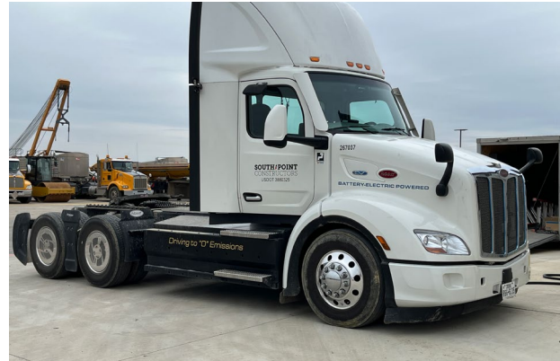
We partner with equipment providers to field test new technologies, like this Peterbilt 579EV piloted on a transportation project.
